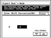
3 Fold the printed test pattern perpendicularly to the paper feed direction, check that there is no shift in the up-and-down direction of the black reference line, and then touch [Enter].
